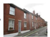
The terrace has slated roofs and brick chimneys stacks, although these seem to be lost at Nos 49 and 50. Two over two sash windows at first floor, and ground floor at Nos 49 and 50, but Oxford type sashes to the ground floor of the remainder. These all appear original. The entrance doors are generally modern except at No 49. All openings have stone lintols, two of which are painted at No 49.
