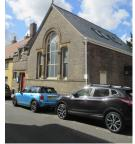
To the north is a modern extension presumably from the 1970s which is the reception for the building's current user. This is set behind a boundary wall with a small car park area. The extension is in a sand faced fletton, which rather lets it down as otherwise it is an entirely 1970s design not compromising to its location and another element adding to the mix of styles in the street.
